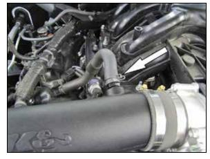
11. Connect the factory crank case vent hose to the fitting installed into the K&N<sup>®</sup> intake tube and secure with the factory spring clamp.
