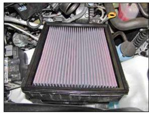
6. Install the K&N<sup>®</sup> air filter into the lower air filter housing and then reinstall the upper housing. Do not secure the lid at this time.
