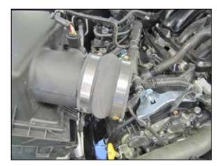
7. Install the provided hump coupler (08171) onto the factory air filter lid and secure with the provided hose clamp.
