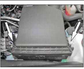
5. Release the two clips securing the upper air filter housing and then lift up the housing and remove the factory air filter.
